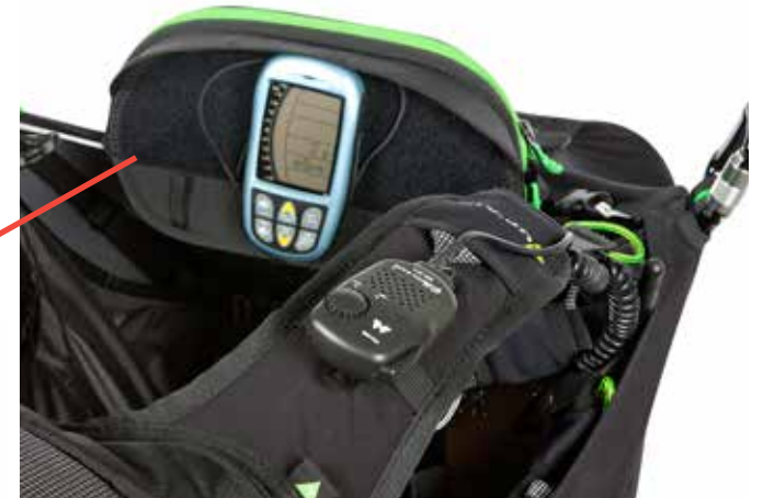
3 Cockpit with removable instrument support.
