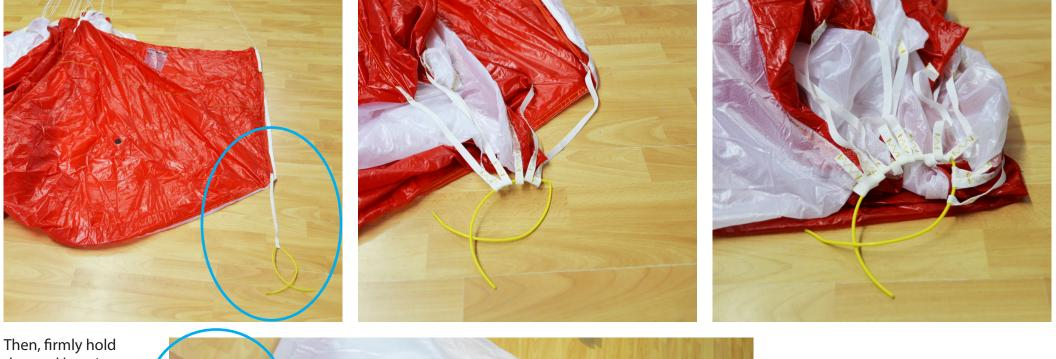
Then, firmly hold the cord keeping the lanyards tightly assembled together.
