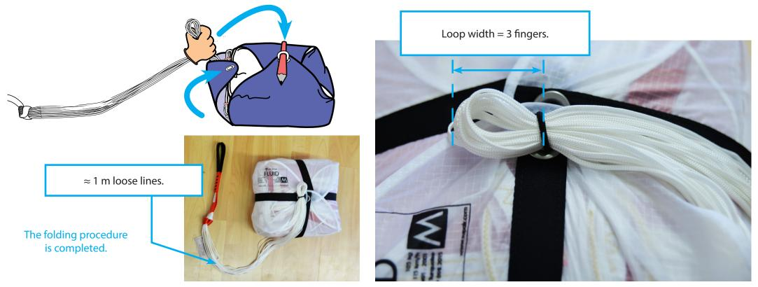
Make sure that all the equipment needed for the packing procedure is accounted for, and that none of it was mistakenly left inside the folded parachute.
