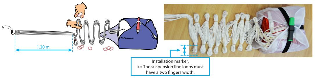
Tuck away the coiled lines inside the space in front of the canopy while keeping a 1.20m line length for the subsequent outer coiling.
