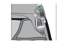
7. Tuck away the risers excess ( without making knots ) under one single flap :
