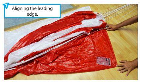
b. Follow the leading edge to find the second panel. This panel is laid out flat in one motion, and rectangular shape.
