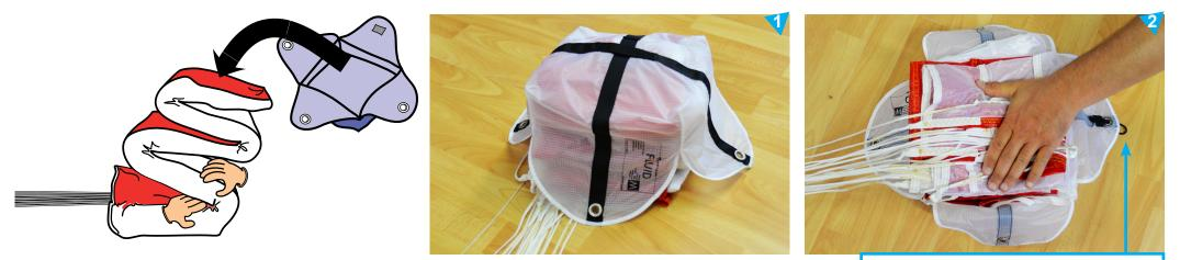
Position the POD's elastic loop opposed to the suspension lines.
