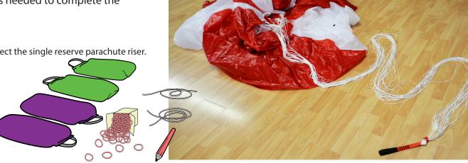
b. Attach the parachute on a fixed point to keep it stretched and under tention.
