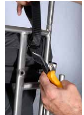
The use of a screwdriver to pivot the buckle, and a pair of pliers to pull the strap can be helpful to simplify the task.
