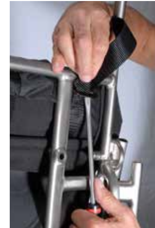
The use of a screwdriver to pivot the buckle, and a pair of pliers to pull the strap can be helpful to simplify the task.
