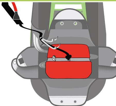
**1.** Place the risers « J » under flap « A ». Push them through between flap « B » and the upper flap in order to stow away the riser and lines excess from the reserve « K » to the bottom of the pocket.
