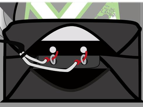
**3.** Close and secure the assembly by pushing the safety pins in their respective receiving loop-cords, then tidying up the handle bridle between flaps « B » and « C », maintain it in place with the help of the upper « C » flap stitched strap.
