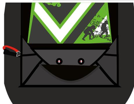
**4.** Tuck away the remaining upper flap end into the receiving neoprene pocket located on the lower flap, and fix the handle to the Velcro® in order to tidy up the assembly.
