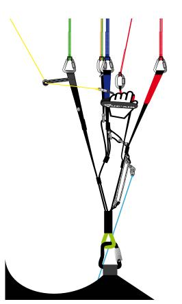
To reopen the "Ears", bring the accelerator/speedbar back to its neutral default setting, then let go the risers symmetrically. You can pump the brake/toggles on either side of the wing to facilitate its reopening sequence.
