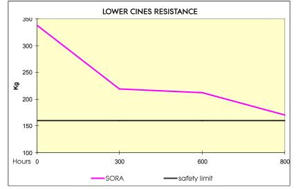
Values in the graph above show an average of measurements taken on our test sample. On some SORA gliders with more than 1,000 flights the readings on lower lines were more than 200kg, well above the 160kg safety limit.
