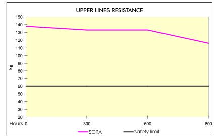
Resistance levels on upper lines throughout the life of a glider remain well above safety requirements. Even after 800 hours, the lineset of our test sample displayed values of double the safety limit (120kg vs 60kg).
