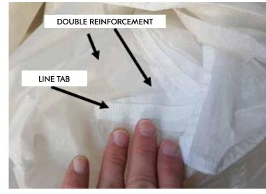
Anchors for line attachments have been generously proportioned in order to ensure structural stability of the glider over time. They are further strengthened by a double reinforcements of the cell wall.
