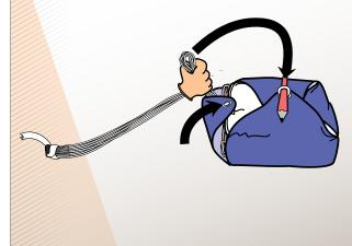
17. Coil the remainder of the lines on the outside of the reserve parachute container.
