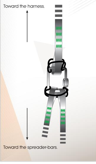
**2.** Connect the risers atop each spreader-bar (main hooking location), with the rectangular lnox (stainless steel) Maillons + the flexible elastic rings.
