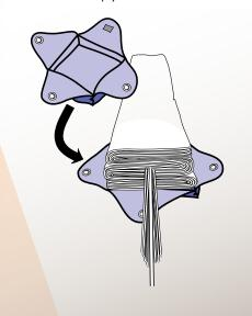
13. S-fold the canopy into the container, leaving a small space for the lines to be coiled in.
