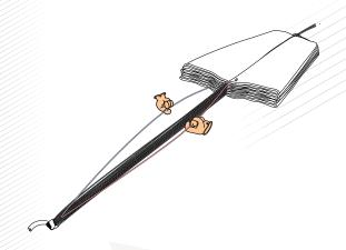
10. S-fold the left side of the canopy under the centre of the chute, then S-fold the right side of the canopy onto the centre of the chute. Keep the canopy neatly folded using sandbags / books.
