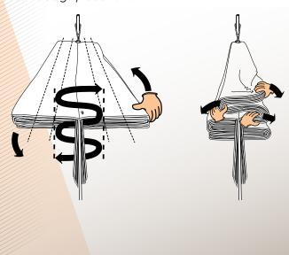
11. Release the tension on the canopy and IMMEDIATELY remove the tie holding the folding loops together. For safety reasons, this procedure should ensure that this tie cannot be inadvertently left in place on the folded chute (SEE inventory list).
