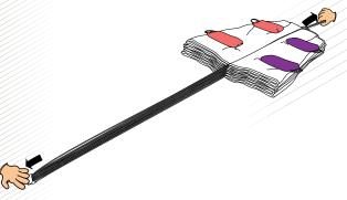
6. Successively arrange all the panels on the right, one on top of the other. Repeat this process with the panels on the left side, starting with panel 1.
