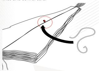
**b.** Bring the chimney top downward by pulling the APEX line to the cord level.
