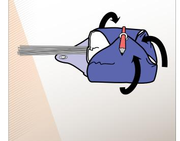
15. Coil the lines into the accommodating space left for them, leaving about 0.5 to 1m length of lines outside for the outer coils.
