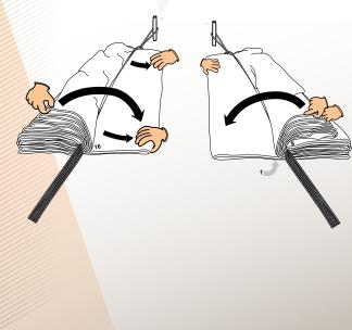
7. Ensure that the number of panels on each side is identical and matching with the total amount of panels of the SPECIFIC model. Take time to verify that the bottom of the skirt (leading edge) is perfectly aligned.
