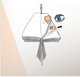
9. Control both lower and upper lines, ensuring that they run freely from the canopy to the riser(s).
