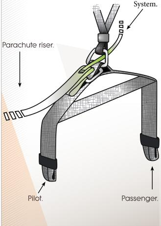
**3.** 3 / On both sides, push the small recoil » André Rose « strap / webbing, through the main paraglider carabiner riser, and connect it to the « B « or « C « paraglider riser using a triangular ( Delta shaped ) Maillon - riser denomination can vary from manufacturer to manufacturer.
