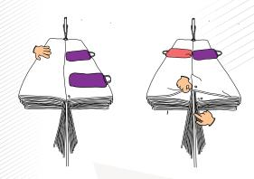
8. Lift the upper line to make sure that the folds are tidy along the whole length of the panels and that the wind channel is unobstructed right up to the apex of the canopy.
