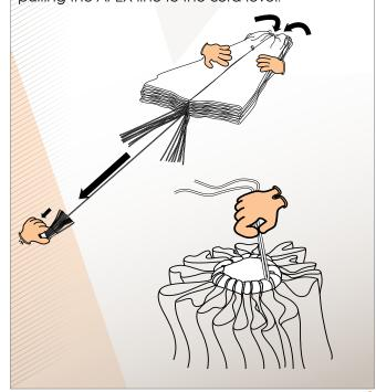
5. Separate the two outer lines (the outside lines on the riser) and lay them on the comb. Flake the canopy, starting with the lower panel on the right (panel 16), arranging it neatly.
