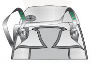
2. Connect the risers to the parachute with a rectangular 7 mm stainless steel (Inox) Maillon Rapide. Use the flexible elastic rings to secure the bridles to the Maillons as indicated below.
