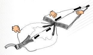
3. Even out the parachute into a pine tree shape while holding the webbing and stretching out the central cord.
