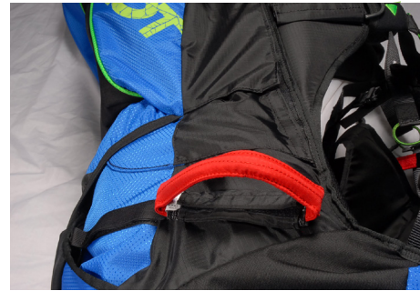
Handle positioning in its holding sleeve.
