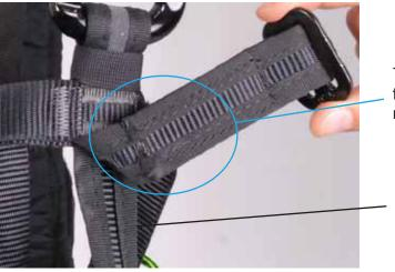
The purpose of repair is to protect the structural strap from the wear caused by the end of the "webbing return" (blue circle).
