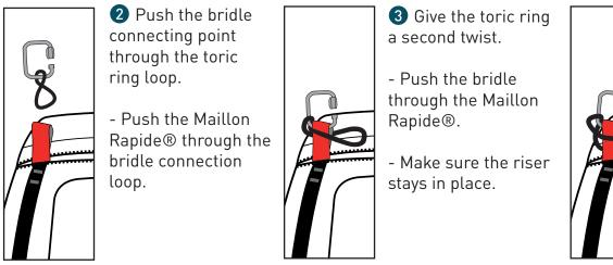
Close the Maillon Rapide® by hand, then tighten using a set of pliers and making a 1/4 turn.
