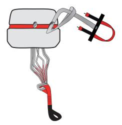
Tighten the handle/POD connection securely.
