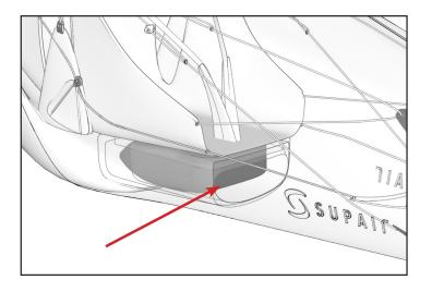
Insert the Inflatable BUMP by first passing the pipe through the hole at the bottom of the pocket on the top right. The passage (8mm diameter hole may be difficult to find)
