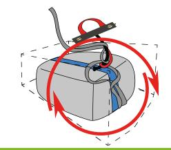
If the emergency parachute does not have a snug fit inside the rescue pocket, it could potentially rotateon itself while using the harness. The risers then roll up around the rescue parachute pod handle and prevent a deployment.
