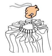
**4.** Control both lower and upper lines, ensuring that they run freely from the canopy to the riser(s).
