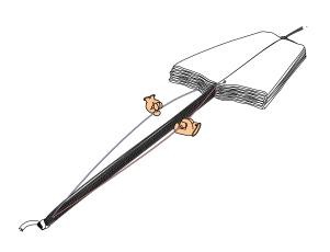
9. S-fold the left side of the canopy under the centre of the parachute, then S-fold the right side of the canopy onto the centre of the chute. Keep the canopy neatly folded in place using sandbags or books.
