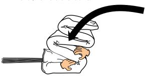
12. Place the pod at the top, then flip it all upside down with the "S" folded parachute. Keep a small space at the front of the parachute's leading edge to later fold and tuck away the lines.
