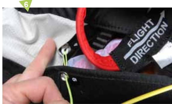
Push the end of the cord through the elasticated loop #4, then guide it through the grommets #5 and #6
