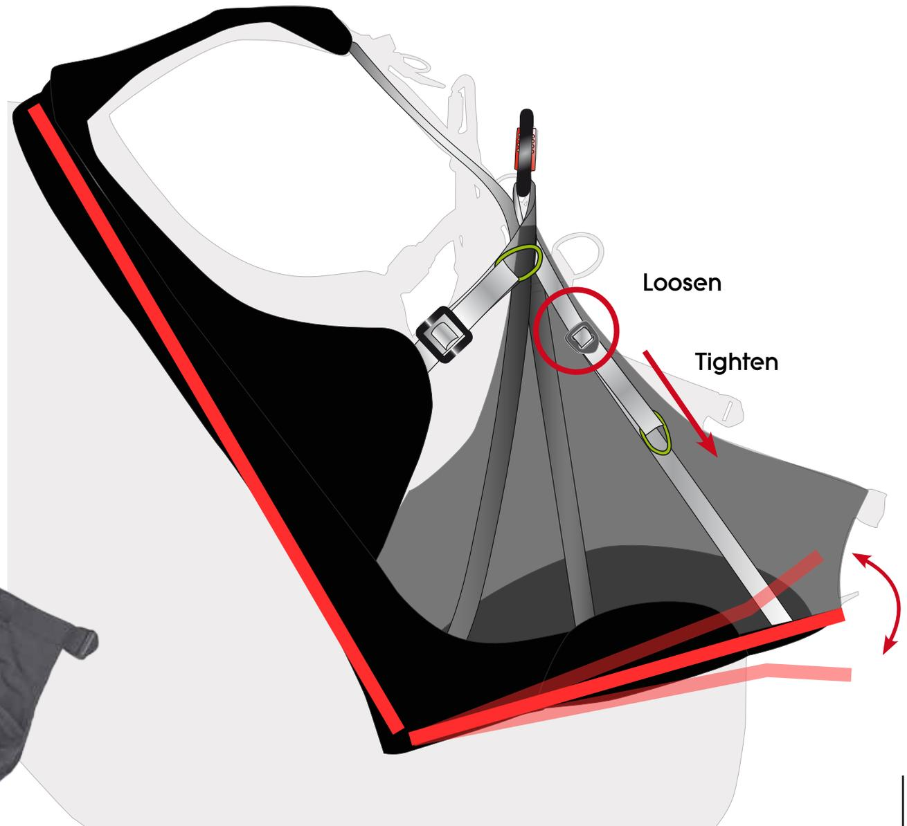
How to turn the Altirando2 harness mode into the backpack mode:
