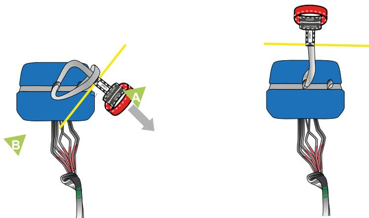
1. Place the handle inside the middle webbing loop and make a lark's head knot with the handle.
