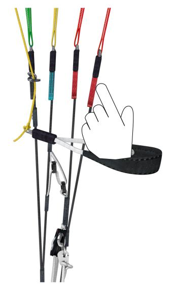
To reopen the "Ears", bring the accelerator/speedbar back to its neutral default setting, then let go the risers symmetrically. You can pump the brake handles on either side of the wing to facilitate its reopening sequence.
