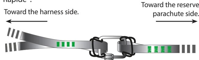
2. Connect the riser split side to the harness's shoulder attachment points using the provided stainless steel (Inox) 6 or 7 mm.
