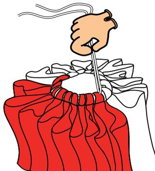
**4.** Control both lower and upper lines, ensuring that they run freely from the canopy to the riser(s).
