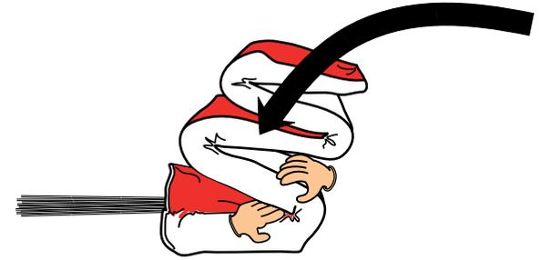
12. Place the pod at the top, then flip it all upside down with the "S" folded parachute. Keep a small space at the front of the parachute's leading edge to later fold and tuck away the lines.
